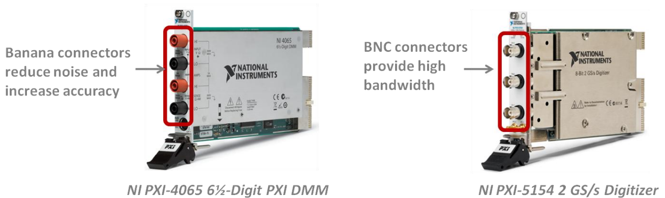
Figure 4. DMM connectors are optimized for accuracy. Digitizer connectors are optimized for bandwidth.
