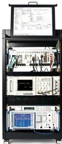
Figure 4. Example of a Hybrid Test System Based on PXI, LAN, and USB Instruments
