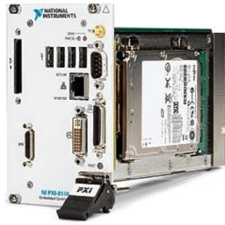
Figure 2. NI PXI-8110 Core 2 Quad Q9100 2.26 GHz Processor Embedded Controller: Notice the familiar PC peripherals such as keyboard/mouse and monitor connections as well as the hard drive, USB 2.0, Ethernet, serial, ExpressCard, and other standard PC peripherals.
