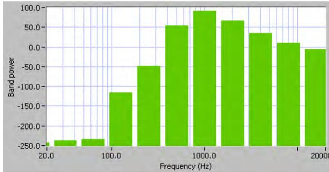
Figure 22. Octave analysis groups frequency bands on a logarithmic scale to emulate how humans perceive sound.
