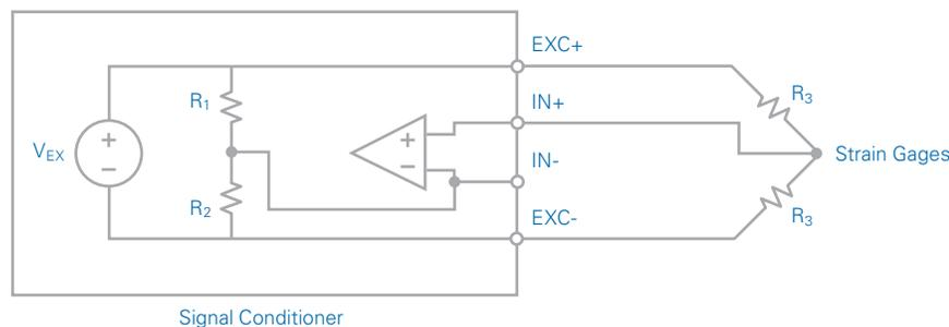
Figure 7. A signal conditioner provides excitation and bridge completion for a half-bridge strain gage circuit.
