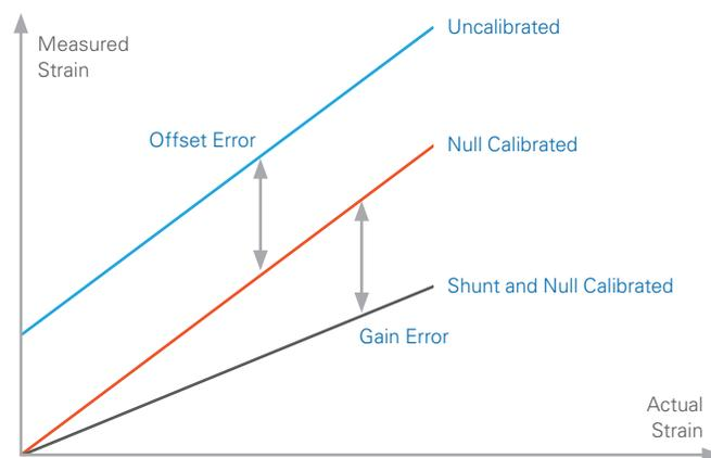
Figure 11. Null and shunt calibration adjust the offset and gain error of the measurement device.
