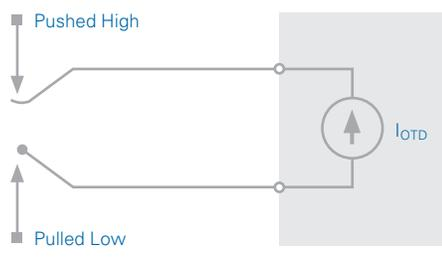
Figure 6. The open thermocouple detection circuit pushes the voltage high when the thermocouple breaks.
