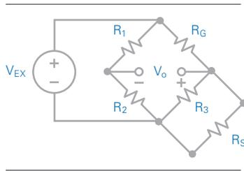
Figure 12. Shunt Resistor Connected Across  $R_3$
