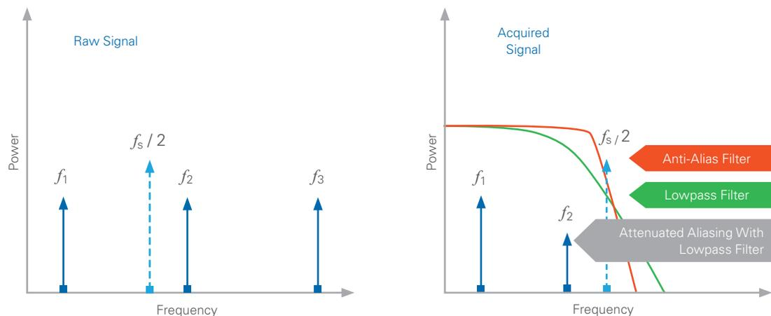
Figure 14. Anti-alias filters with steep roll-off help attenuate noise just above the Nyquist frequency.
