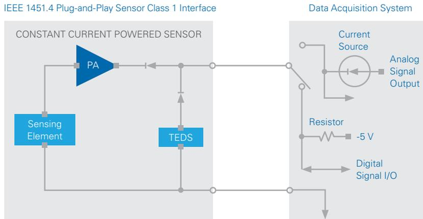
Figure 24. This Class 1 two-wire interface multiplexes analog measurement and digital TEDS data.
