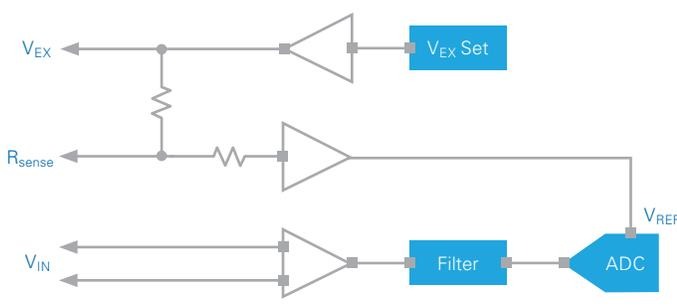
Figure 8. A ratiometric design uses excitation voltage as a reference to ADC to correct for unstable power sources.
