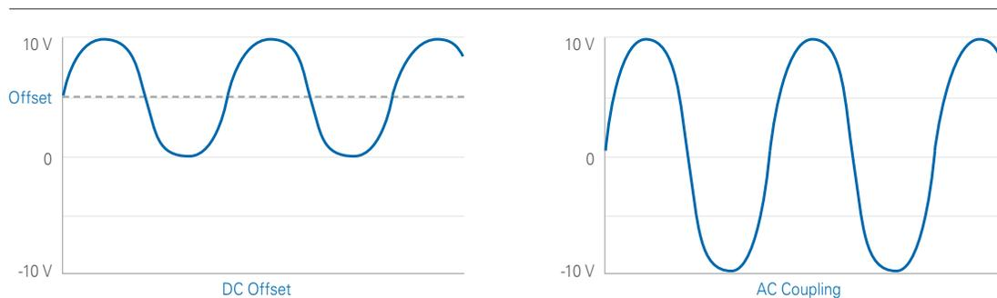
Figure 13. AC coupling filters out the DC component of a signal to increase measurement resolution.
