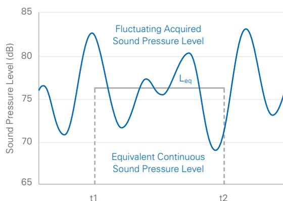
Figure 15.  $L_{\text{eq}}$  is used to quantify long-term exposure to sound in a given environment.
