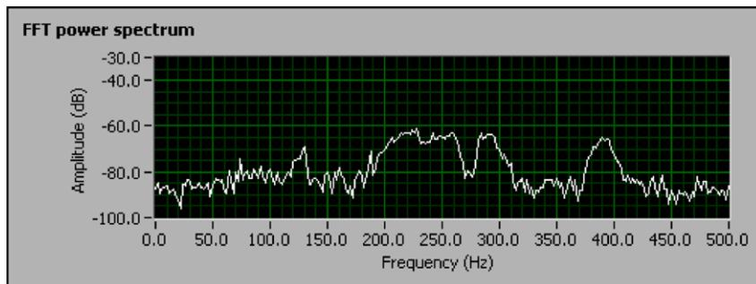
Figure 20. The FFT power spectrum shows no peaks as the rotational speed of the fan changes.
