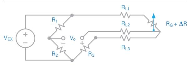
Figure 9. 3-Wire Strain Gage Configuration
