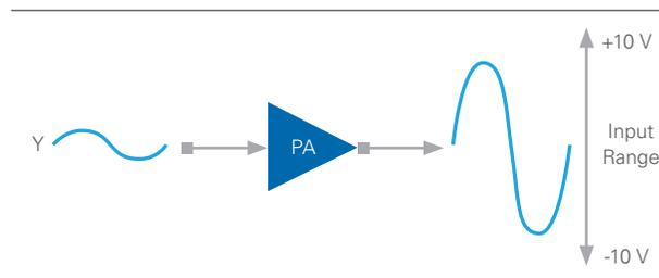
Figure 3. Amplify thermocouple outputs to detect smaller signal changes and use the full ADC input range.
