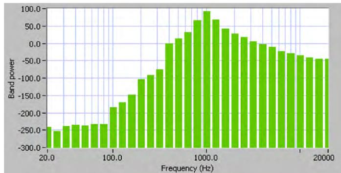
Figure 23. Fractional octave filters provide higher resolution.
