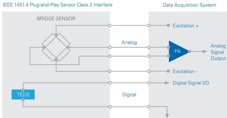
Figure 25. This Class 2 multiwire interface enables plug-and-play functionality.
