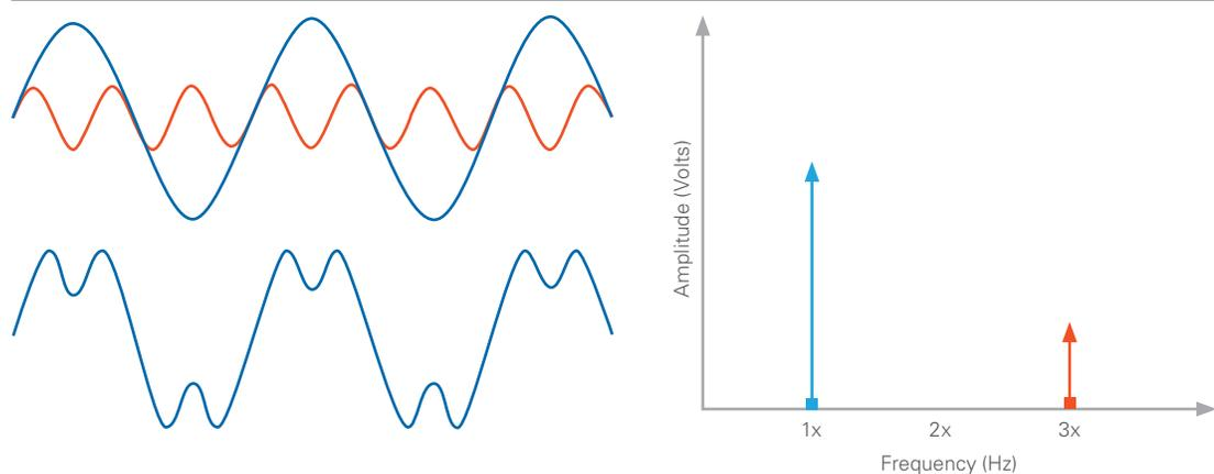
Figure 16. The frequency spectrum shows different amplitudes and frequencies of sinusoidal components.
