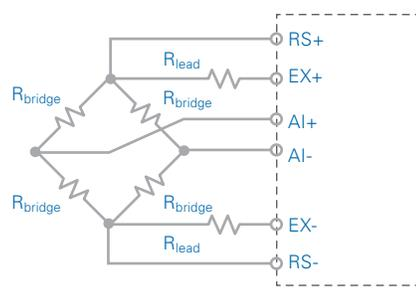
Figure 10. Remote sense measures the actual excitation voltage delivered to a bridge over long distances.
