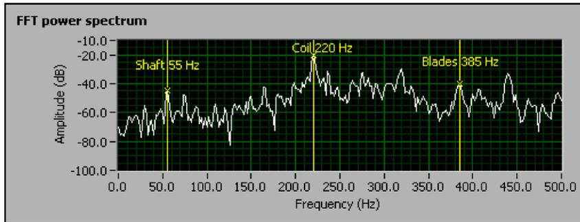
Figure 19. Frequency Components of a PC Fan Vibration Signal
