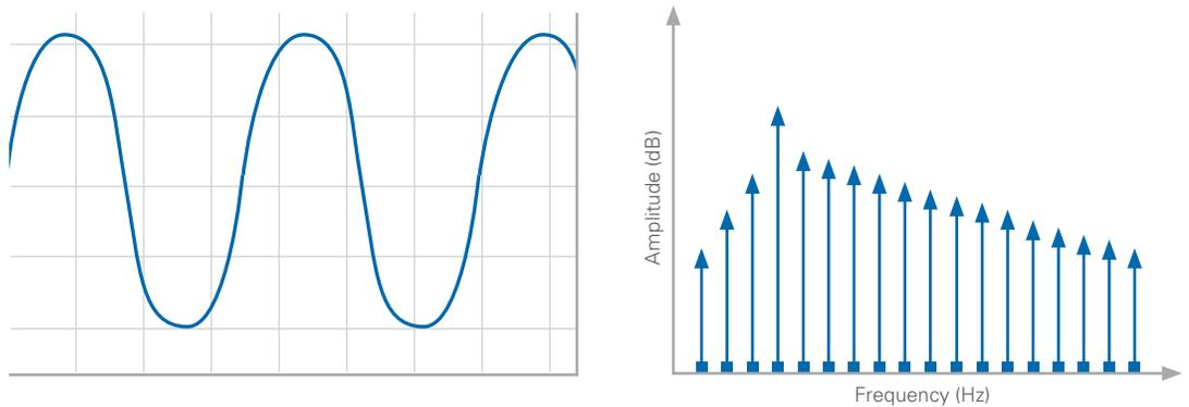
Figure 17. Measuring a noninteger number of periods results in spectral leakage in the frequency domain.
