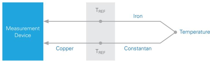
Figure 4. Cold-junction error adds more voltage to a thermocouple measurement.
