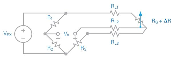
Figure 9. 3-Wire Strain Gage Configuration
