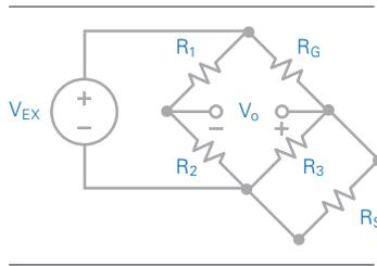
Figure 12. Shunt Resistor Connected Across R3
