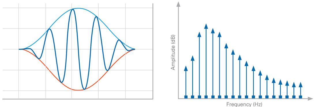
Figure 18. Applying a window minimizes the effects of spectral leakage.
