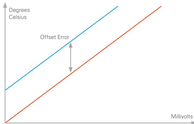
Figure 5. Autozero compensates for offset error.
