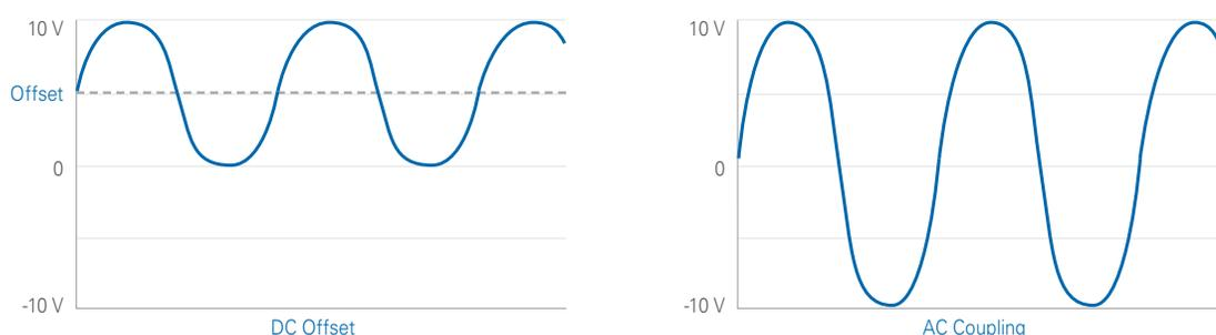
Figure 13. AC coupling filters out the DC component of a signal to increase measurement resolution.
