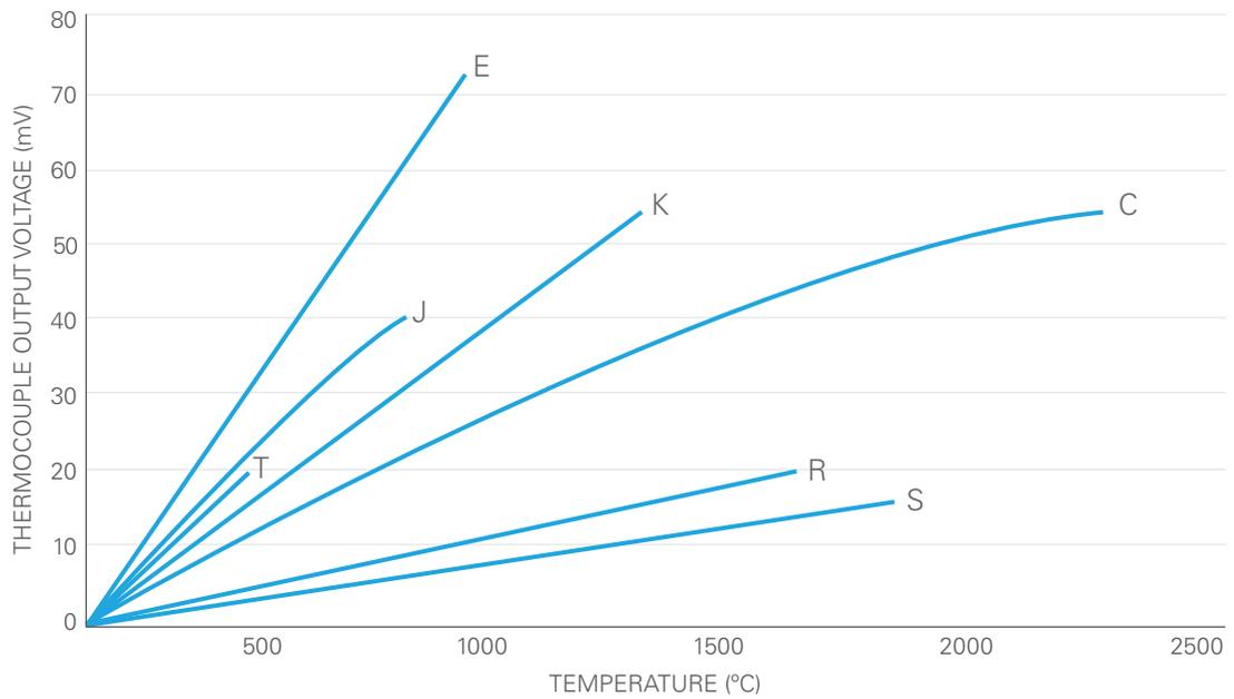
Figure 1. Thermocouple Output Voltage Versus Temperature<sup>1</sup>
