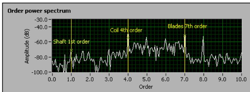
Figure 21. Order power spectrum identifies peaks by normalizing rotational speed.
