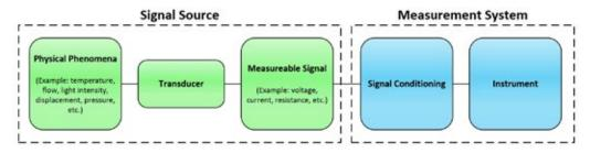
Figure 1. A signal source is fed into a measurement system that comprises an instrument and signal conditioning.
