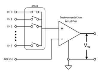
igure 5. An NRSE instrument's common point is the voltage provided at the negative terminal of the instrumentation amplifier.
