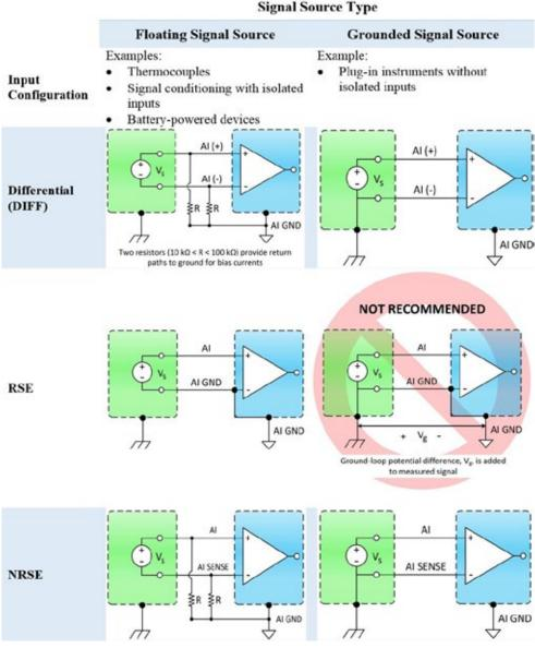
Figure 8. Instrument Configuration Versus Signal Source Type Summary.
