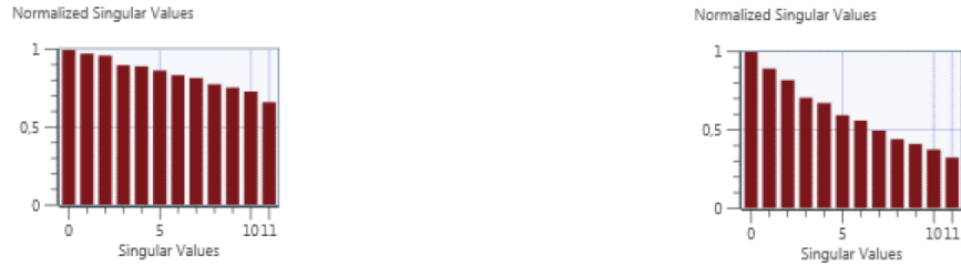
Figure 9-4. MIMO channel singular values at the mobile station (left) and at the base station (right).
