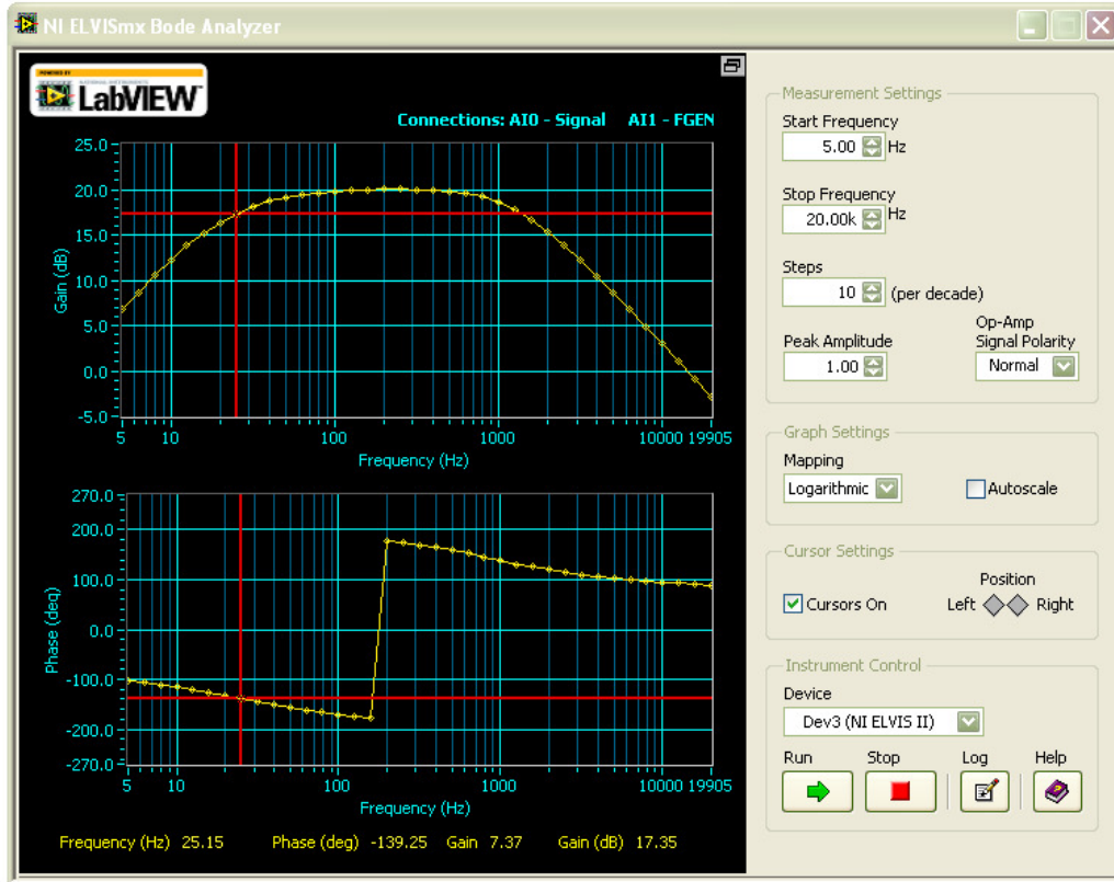
Figure 4.12. Bode Measurement of Bandpass Op Amp circuit
