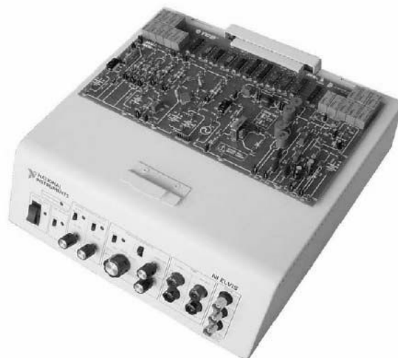
Figure 3 eTCB board interfaced with NI ELVIS workstation 13
