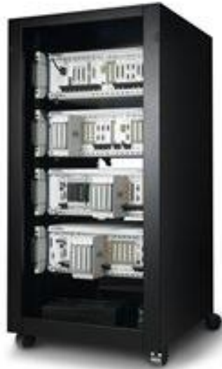
Figure 1. High-Channel-Count Structural Test System
