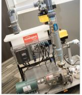
You can manually create shaft misalignment or cavitation on the smart pump demo that holds 30 to 60 gallons of water.
