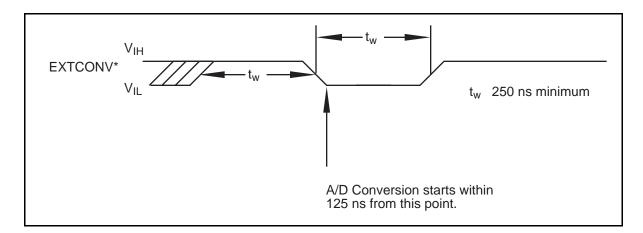
Figure 3-13. EXTCONV\* Signal Timing
