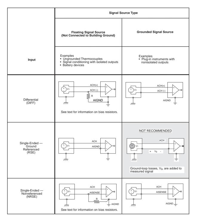
Figure 3-3. Summary of Analog Input Connections
