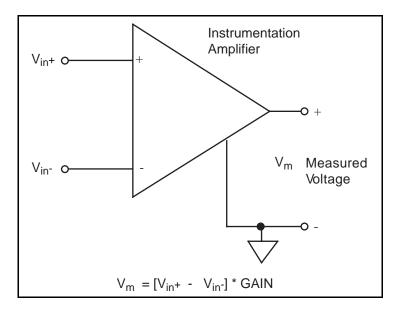
Figure 3-2. DAQPad-1200 Instrumentation Amplifier
