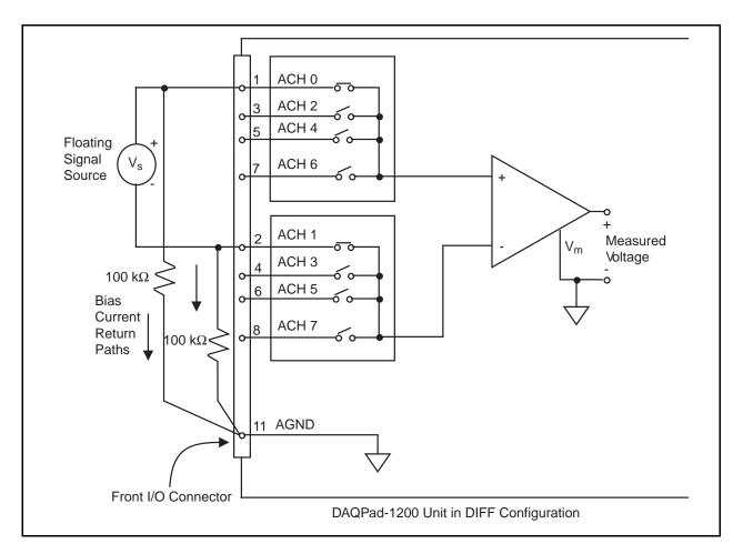
Figure 3-5. Differential Input Connections for Floating Sources
