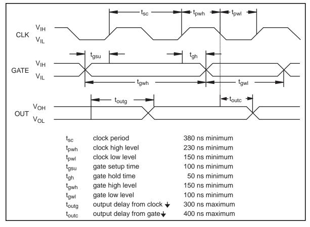
Figure 3-20. General-Purpose Timing Signals
