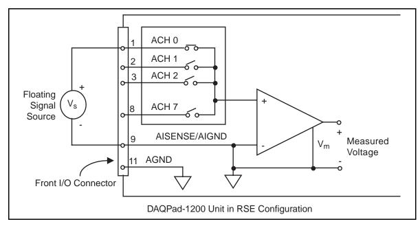
Figure 3-6. Single-Ended Input Connections for Floating Signal Sources
