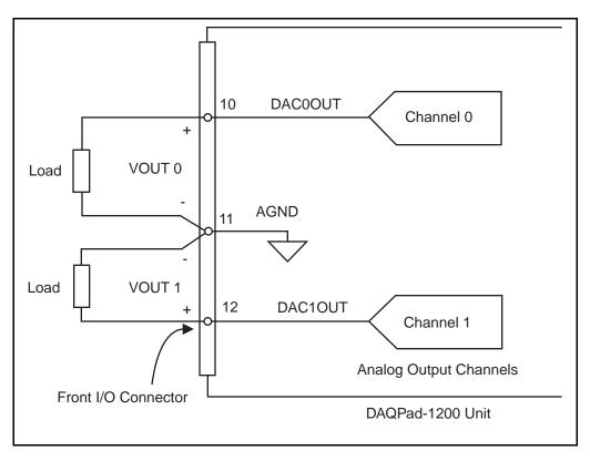
Figure 3-8. Analog Output Signal Connections
