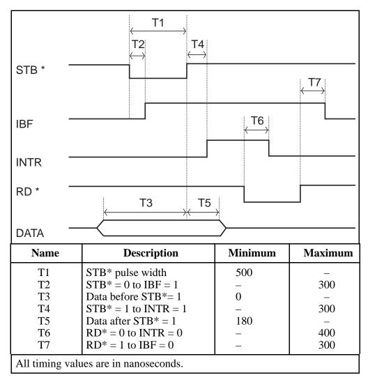
Figure 3-10. Mode 1 Timing Specifications for Input Transfers
