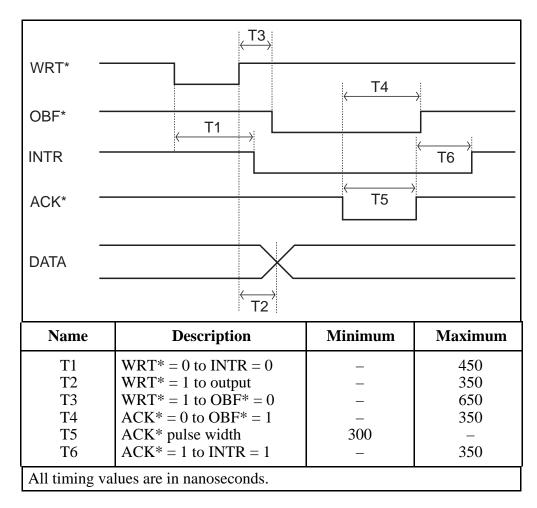
Figure 3-11. Mode 1 Timing Specifications for Output Transfers
