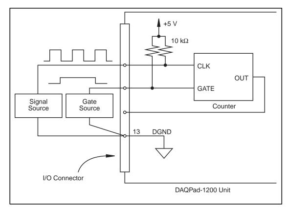
Figure 3-19. Frequency Measurement Application
