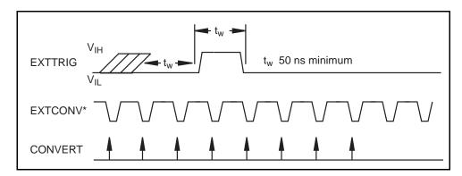
Figure 3-15. Pretrigger DAQ Timing
