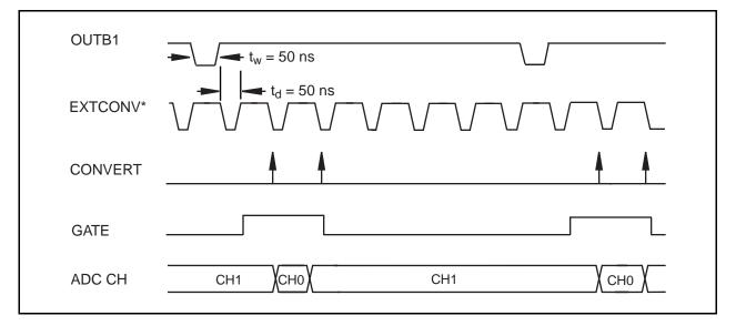
Figure 3-16. Interval-Scanning Signal Timing
