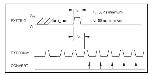
Figure 3-14. Posttrigger DAQ Timing
