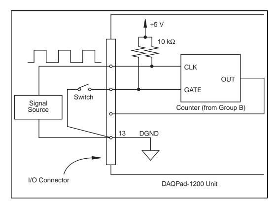
Figure 3-18. Event-Counting Application with External Switch Gating
