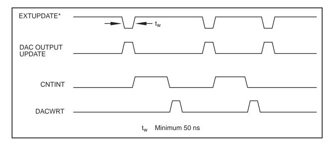
Figure 3-17. EXTUPDATE\* Signal Timing for Updating DAC Output
