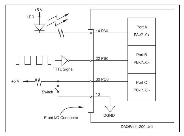
Figure 3-9 illustrates signal connections for three typical digital I/O applications.
