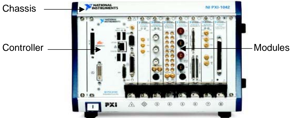
Figure 1. A standard 8-slot PXI chassis contains an embedded system controller and seven peripheral modules.
