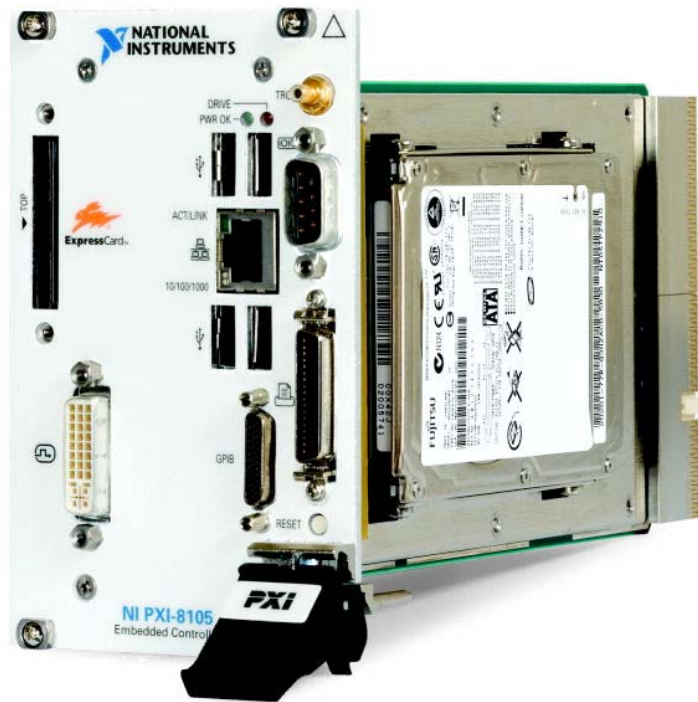
Figure 5. In this photo of the National Instruments PXI-8105 2.0 GHz dual-core PXI embedded controller, notice the familiar PC peripherals such as keyboard/mouse and monitor connections, as well as the hard drive, Hi-Speed USB, Ethernet, serial, ExpressCard, and other standard PC peripherals.
