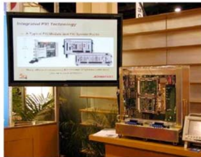
Fig 2 Demo of Mixed-Signal IC Tester Using the PXI Carrier Module (the board in the central transparent case).
