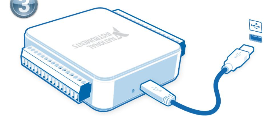
Connect the device to a USB port on your computer. Then connect shielded sensors and signals as described in the user guide.
