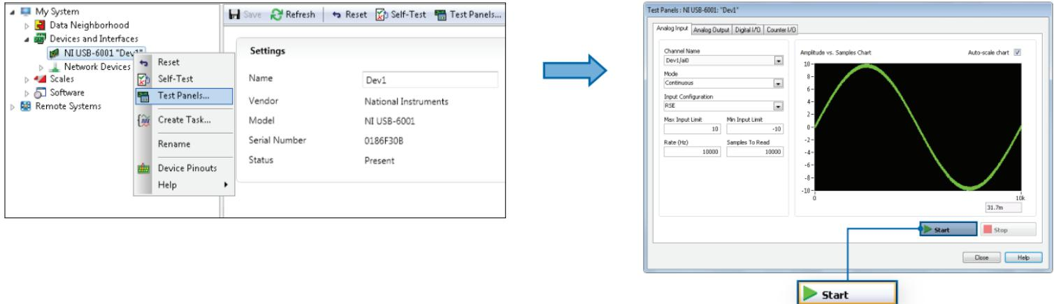
Take your first measurement in NI Measurement & Automation Explorer (NI MAX). Right-click the device and select **Test Panels**. After selecting measurement parameters, click **Start** to verify measurement functionality.
