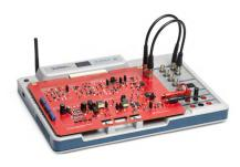
NI ELVIS III WITH THE TI POWER ELECTRONICS BOARD
