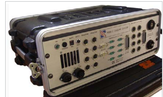
Figure 2. The CCS Mobile Daquire System, Based on the NI CompactRIO Platform
