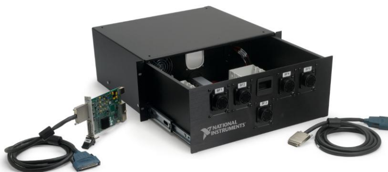
Figure 15: Expansion Drawer for NI ECS-1002
