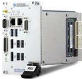
Figure 11: For example, the NI PXIe-8135 controller has the Intel Core i7-3610QE processor, with up to 16 GB of DDR3 RAM, a hard drive, and standard PC peripherals such as ExpressCard, USB 2.0, USB 3.0, Ethernet, serial, parallel and GPIB ports.
