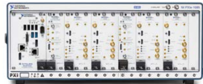
Figure 3. Advanced VRTS Capable of Generating up to Four Radar Obstacles
