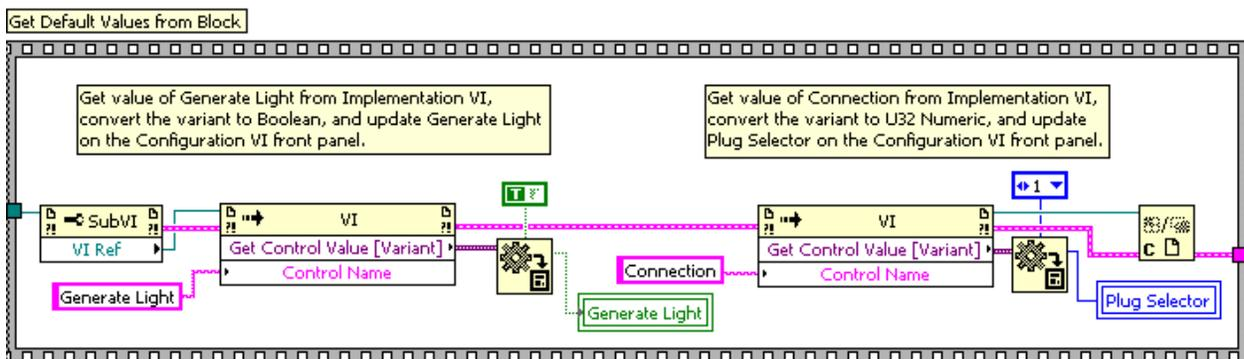
5. Modify the Configuration VI to update the **Generate Light** control on your Implementation VI when a user updates the **Generate Light** checkbox.
