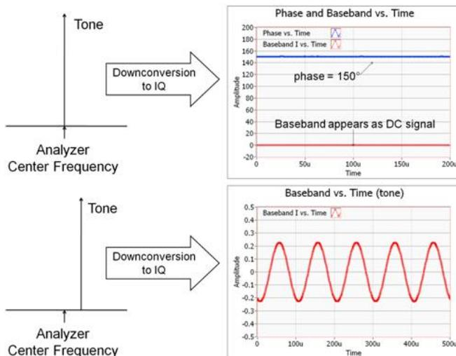
**Figure 5.** Understanding the Effect of Frequency Offset on Baseband Signals
