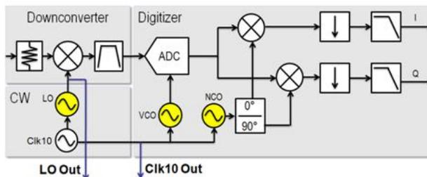
**Figure 4.** Detailed Block Diagram of an NI PXIe-5663 RF Vector Signal Analyzer
