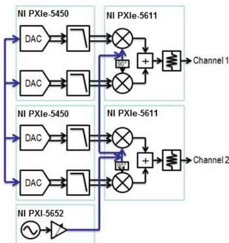
**Figure 2.** Synchronization of Two RF Generation Channels
