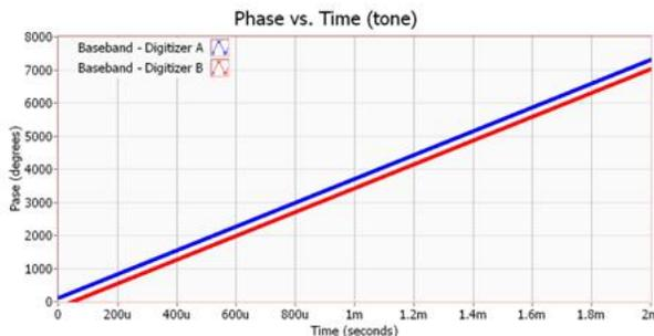
**Figure 6.** Phase versus Time for 10 MHz Tones in an Uncalibrated System
