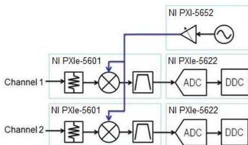
**Figure 3.** Synchronization of a Two-Channel Vector Signal Analyzer System
