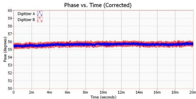
**Figure 9.** Phase versus Time for Calibrated Phase-Coherent RF Acquisition Channels
