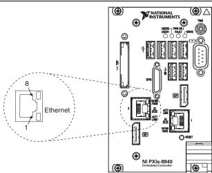
Figure 3-4. Ethernet Connector Location and Pinout
