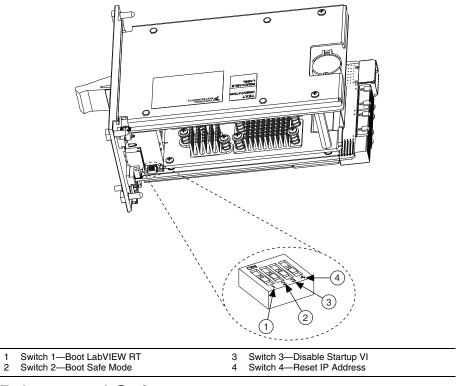
Figure 2-4. LabVIEW RT Configuration Switches
