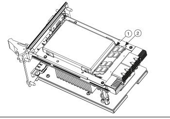
1 DDR3L SO-DIMM Socket
