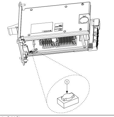
Figure 5-1. Clearing the CMOS Contents
