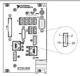
Figure 3-2. DisplayPort Connector Location and Pinout
