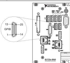
Figure 3-7. GPIB Connector Location and Pinout
