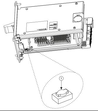
Figure 2-3. Clearing the CMOS Contents
