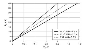
Figure 8. PFI <0..15>/P1/P2:  $I_{ol}$  versus  $V_{ol}$
