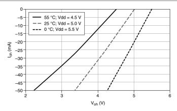
Figure 6. PFI <0..15>/P1/P2:  $I_{oh}$  versus  $V_{oh}$
