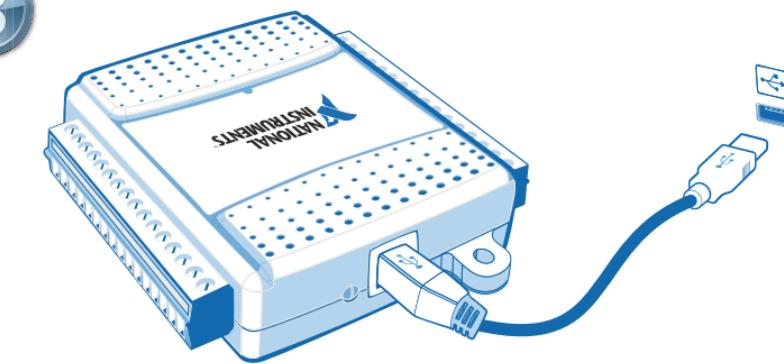
Connect shielded sensors and signals as described in the user guide. Then connect the device to a USB port on your computer.
