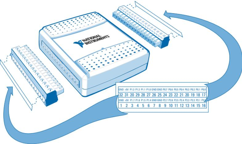
Attach screw terminal connector plugs to device and then apply labels to the connectors.
