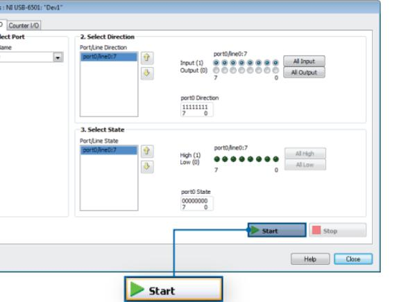
Take your first measurement in Measurement & Automation Explorer (MAX). Right-click the device and select **Test Panels**. After verifying measurement parameters, click Start to verify measurement functionality.
